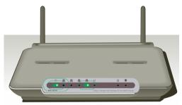
3. Turn on your computers. After your computers boot up, the LAN status LED . on the front of the Modem/Router will be on for each port to which a wired computer is connected. These lights show you the connection and activity status. Now you are ready to configure the Modem/Router for ADSL connection.
